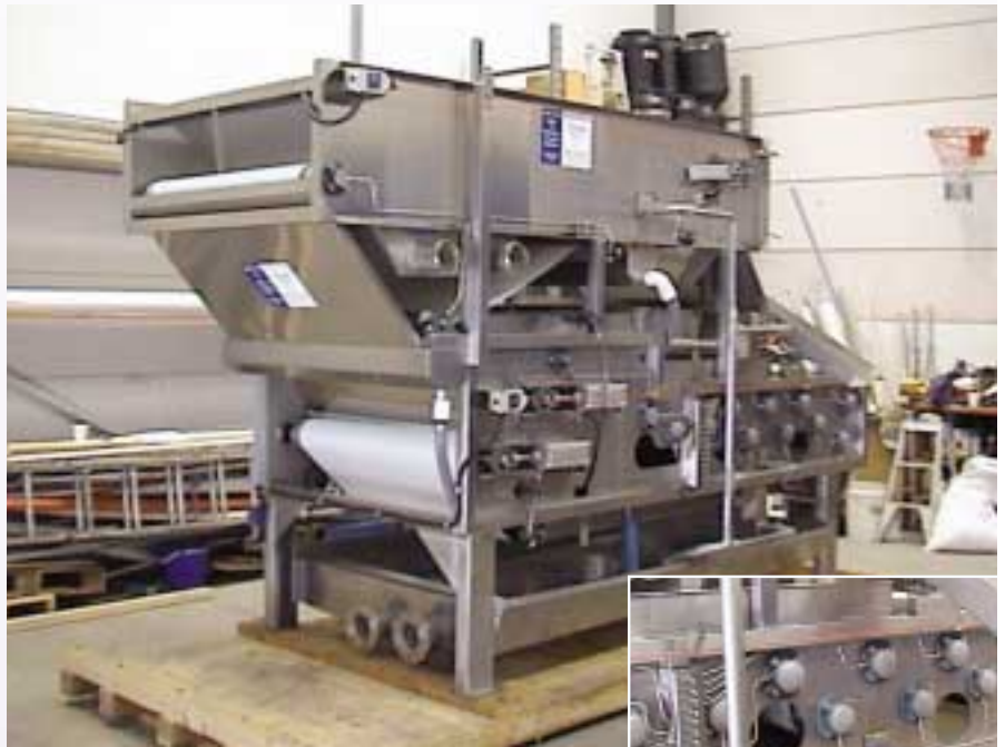
AJM's 9 stage high compression system. (Brad really wanted this picture in so you can see his handy work on the greasing manifold)
